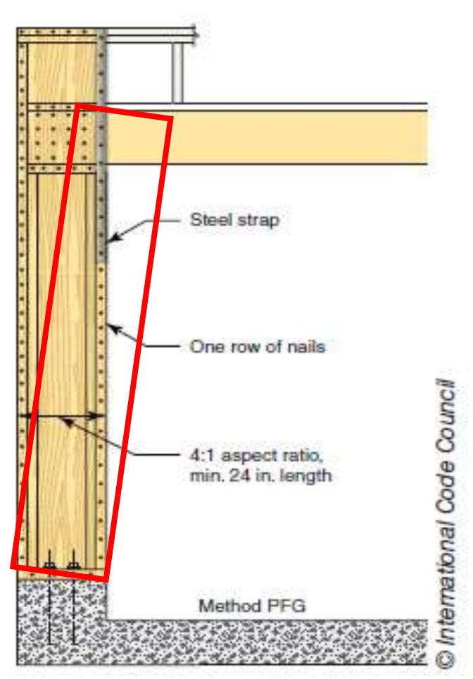
Comparison of nailing of CS-PF and PFG
