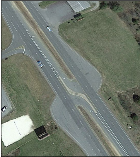
Figure 12. Truck/Emergency Vehicle U-Turn Accommodation (US 74, Whittier, NC)
