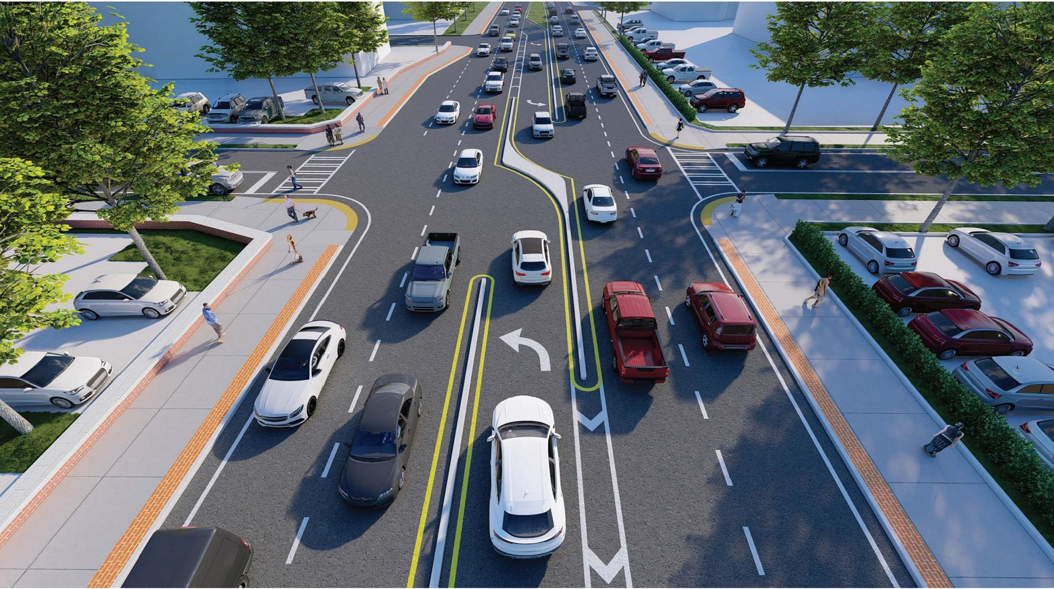
Figure 19. Visual Rendering of Segment Project (RCUT Design)
