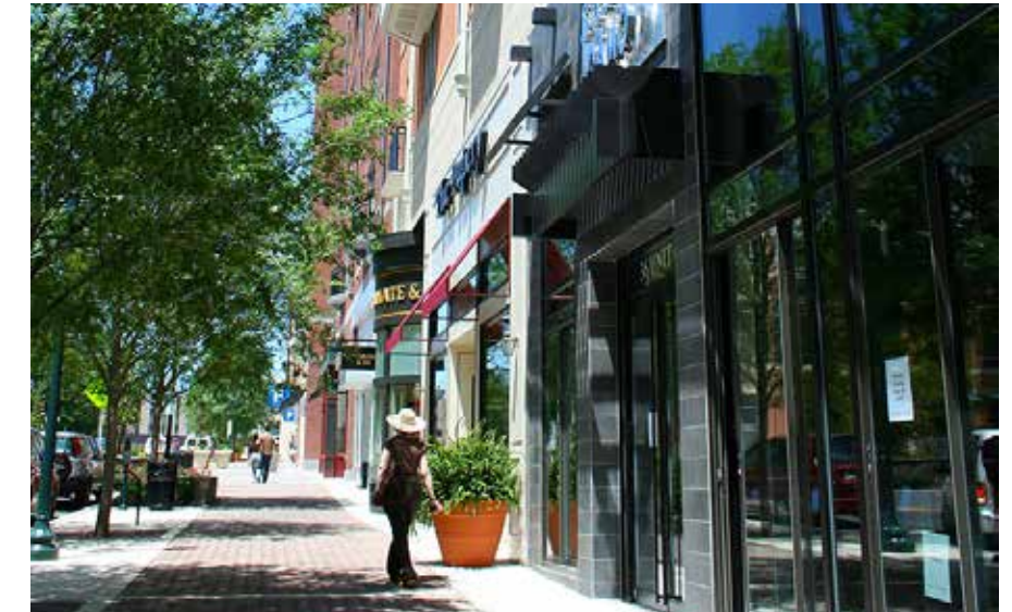
Streetscape with (from right to left) building zone, sidewalks and amenity zone/ planting strip, and parking lane. (Source: Terrain.org)
