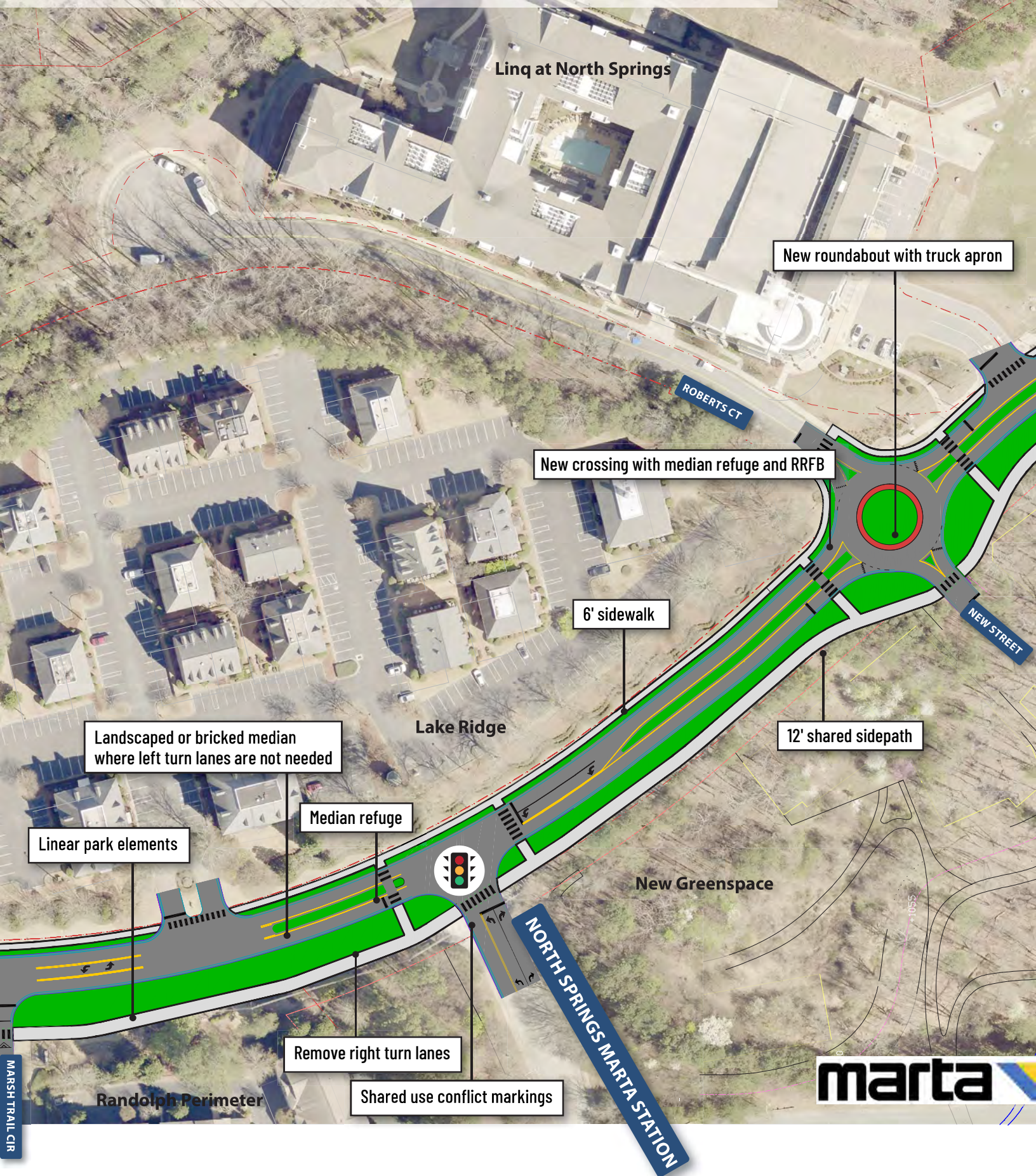
Figure 16 Peachtree Dunwoody Road 10% Concept Design (Peachtree Dunwoody Court to Marsh Trail Circle NE)
