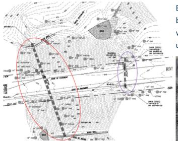
Existing public stormwater pipes were discovered to be failing and in poor condition. Drainage structures were replaced and a "spin-cast" method of lining was used to repair a pipe without excavation.
