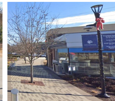
Philips Lumec UrbanScape LED Post-Top on 13.5'ht APR5 Round Aluminum Pole w/ Two-Way Upper and Lower Banner Arms; Medium Gray Textured
