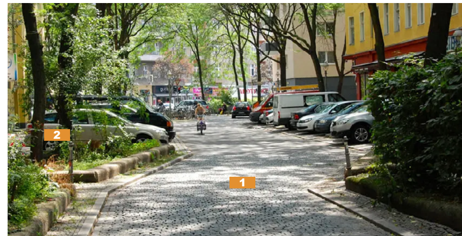
1 Non-linear drive aisle slows down vehicular traffic (4.B.4.-A3) 2 Trees provide shade (4.B.4.-A2)
